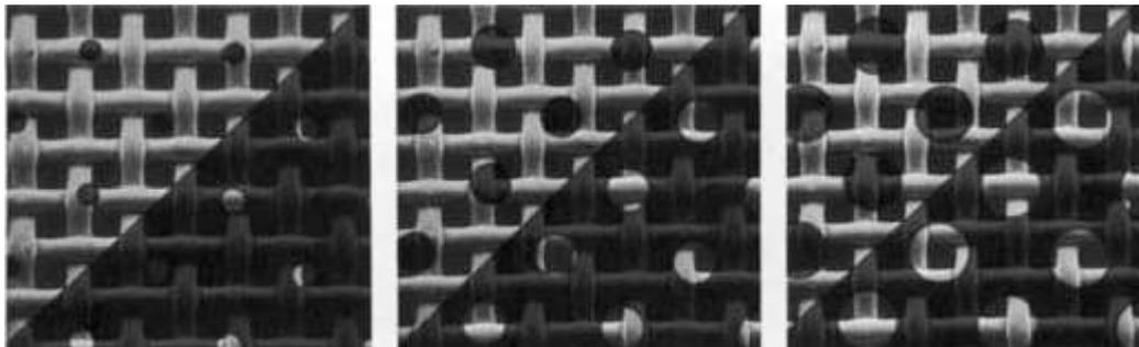
Strictly speaking, the diameter of the smallest half-tone dot on the diapositive should be microscopically measured, in order to select a mesh of the correct fineness.
